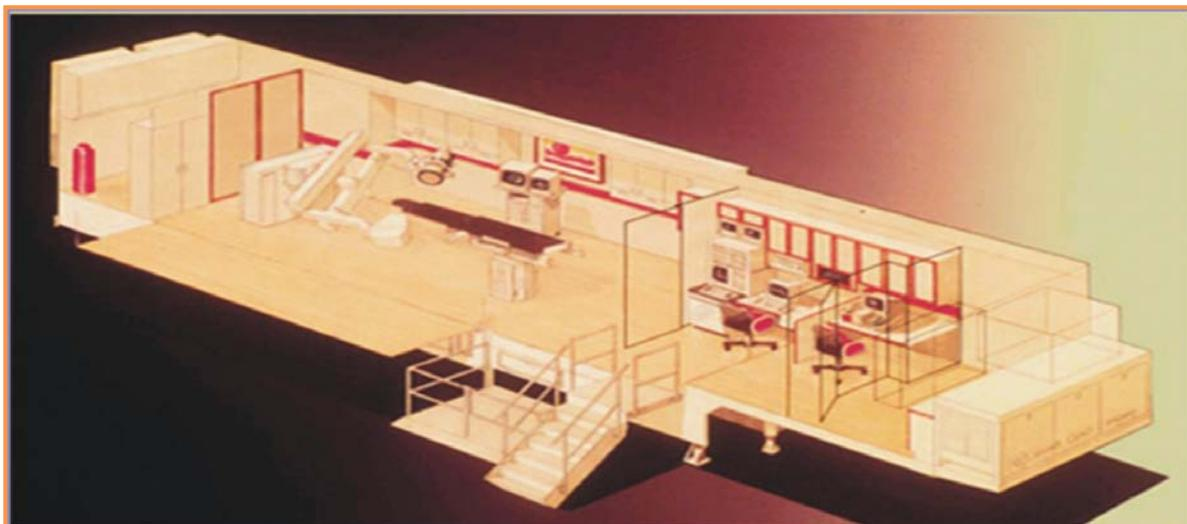
**Fig 2: Mobile Cardiac Catheterization Laboratory Design**
